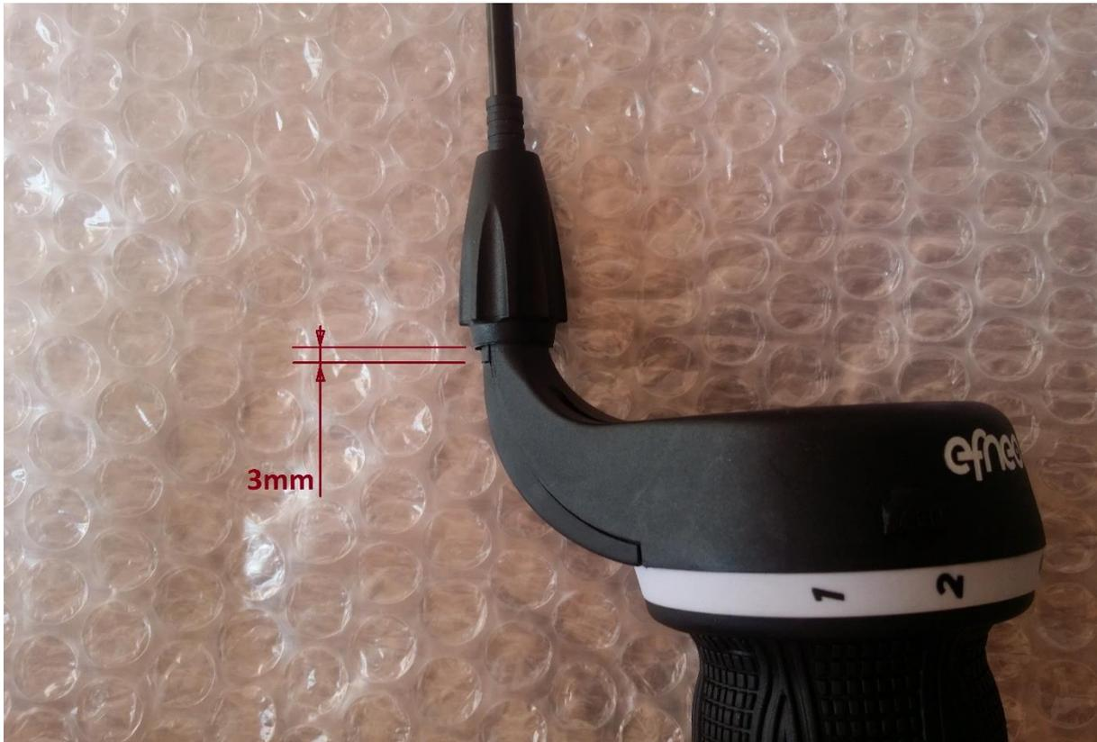
The trigger shifter should have an adjustment barrel in the following position (in the middle of the range):
