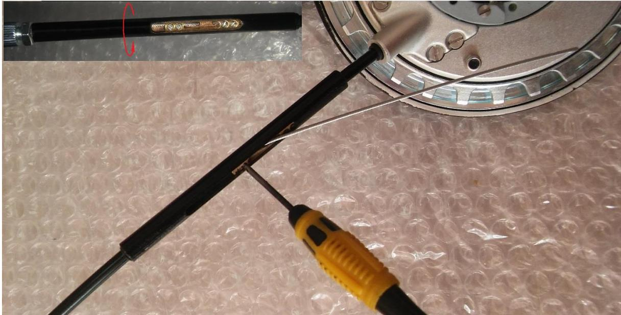
We put a new shifting cable (steel wire should be longer than external housing by at least 5 cm / 2 inches; much longer is OK, too) into the shifter. The shifter has to be in a **3rd gear position**.
