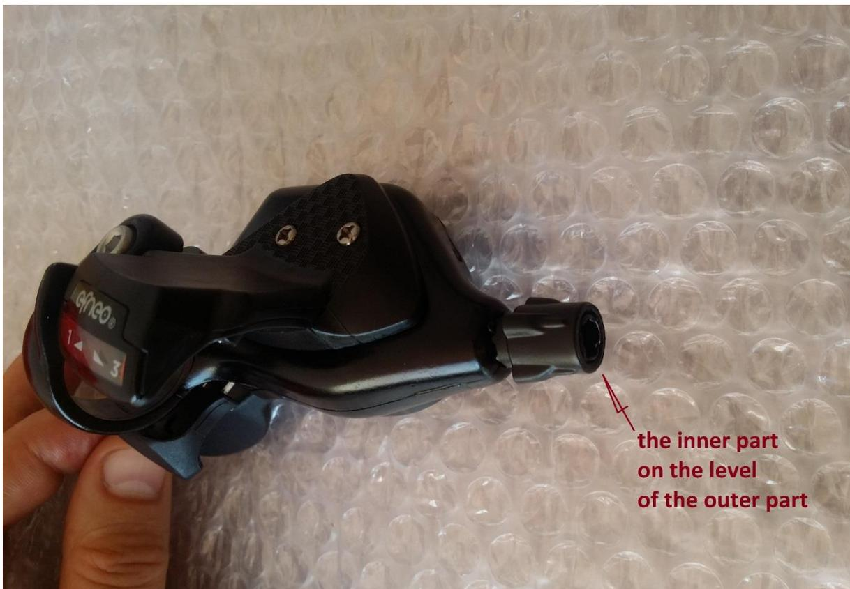
Putting adjustment barrel position to a middle of its range allows for later tuning in both directions!
